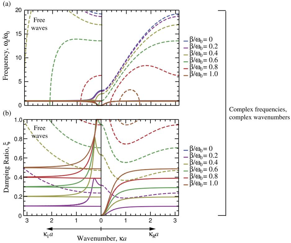
**Fig. 5.** All-complex dispersion curves. The complete frequency (a) and damping ratio (b) band diagrams for free waves generated by the proposed algorithm for all prescribed  $\kappa = \kappa_R + i\kappa_I$  where  $\kappa_R, \kappa_I \in [0, \pi/a]$ .
