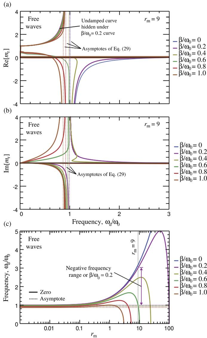
**Fig. 6.** Dynamic effective mass curves. (a) Real component of effective mass; (b) imaginary component of effective mass; (c) zero (solid curves) and asymptote (dashed curves) of Eq. (29) enclosing the region of negative effective mass. The dashed vertical lines in (a) and (b) represent the real and imaginary asymptotes of Eq. (29), respectively. In (c), the negative frequency range for  $\beta/\omega_0 = 0.2$  is highlighted as an example.
